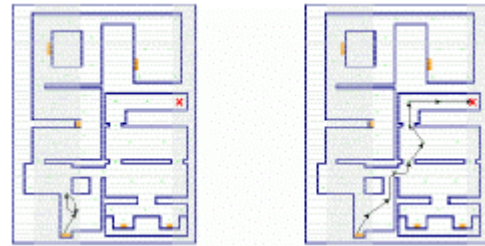
Figure 5. User-specified loop (left) and resulting loop-free learned policy (right).
