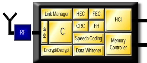
Figure 5: Bluetooth RF and Baseband Controller
